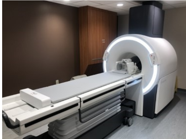
Fig. 7. Photograph taken by Dr. Steven Beyea of Synaptive Medical’s head-only point-of-care 0.5 Tesla magnetic resonance imaging system located in the Biomedical Translational Imaging Centre (BIOTIC) lab at the QEII Health Sciences Centre in Halifax, Nova Scotia, Canada.
