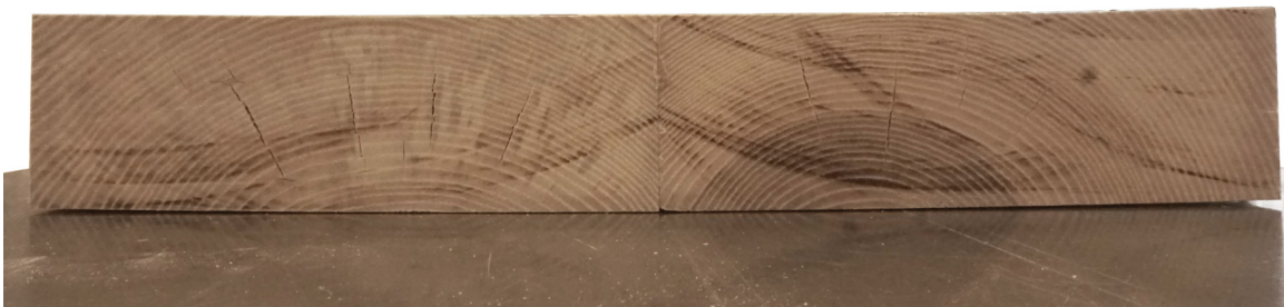
The stool's seat cupped after one day of observation.
