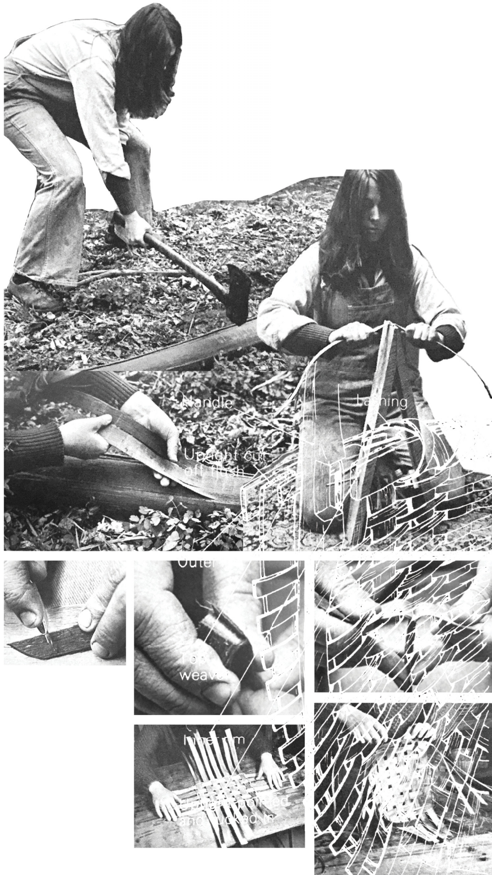
Splints are pounded, halved and finished to be woven into baskets (base images from Fine Woodworking Magazine 1984).
