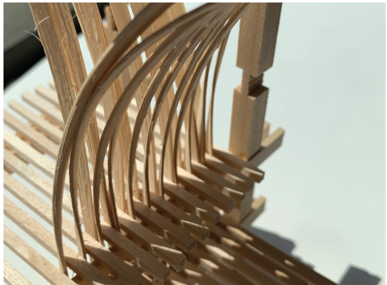
Sketch model exploration of splint to frame connections, using flat reed as a modelling material as a corollary for splints.
