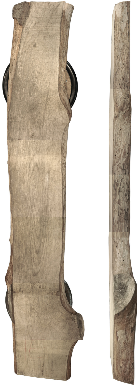
Air dried board acquired for this project through an arborist and woodworker in Fall River, Nova Scotia. This particular board had been infested with the Emerald Ash Borer, evident in the pattern of bore holes left in its bark (right).
