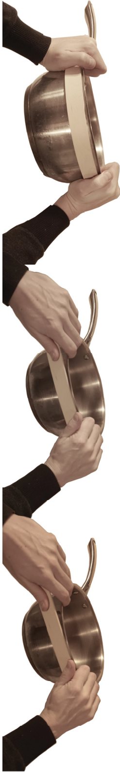
Processes of steam bending using a kitchen pot as simple formwork.
