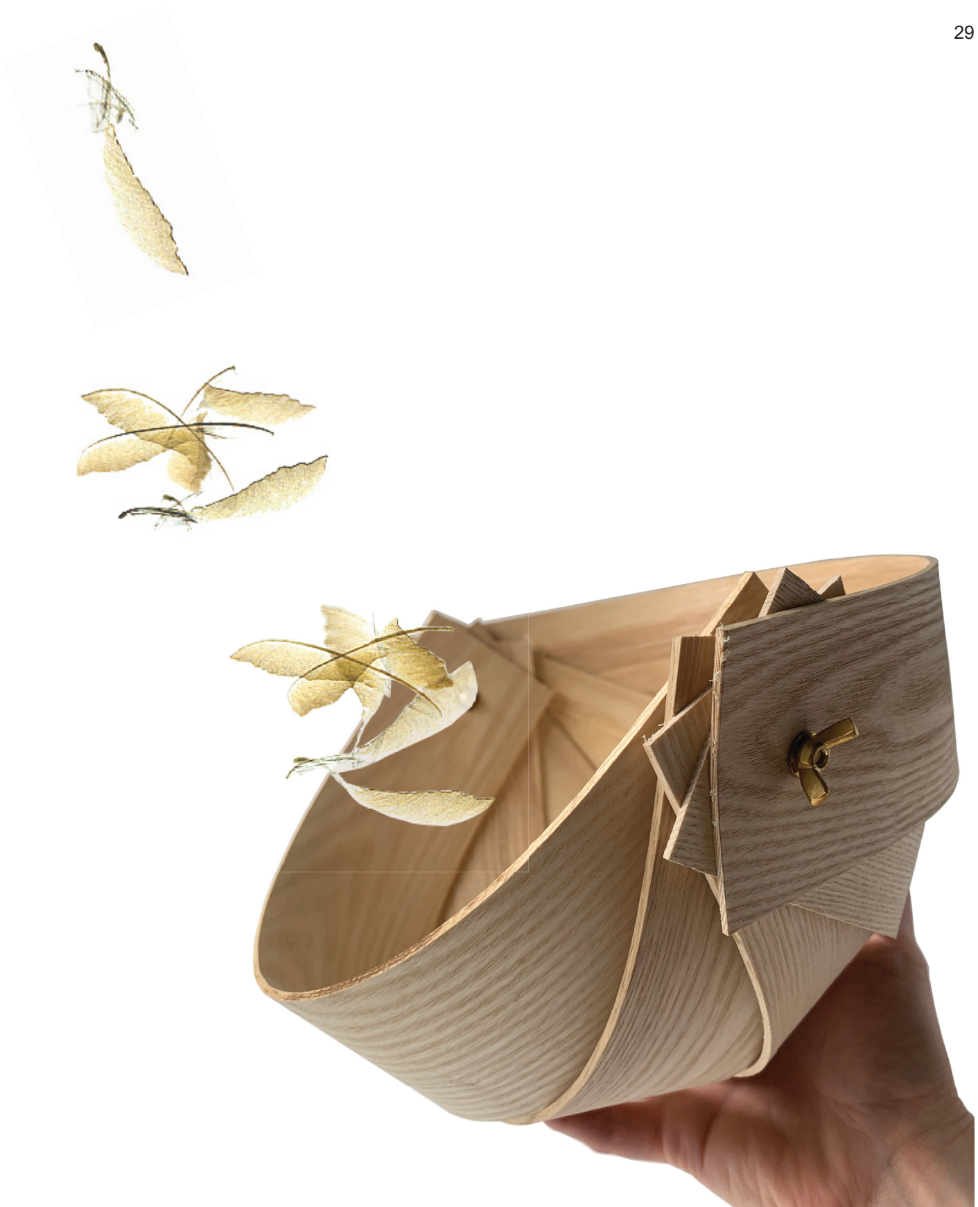
Steam bent ash basket layers \frac{3}{32} " milled components whose bends are incrementally offset and connected with threaded brass hardware.
