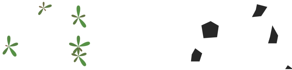
Figure 5.4: Flower glyphs and Polygon glyphs used in this thesis to represent individual participants. Shape of glyphs is indicative of sub-selected features representing individual participant’s smartphone usage. In case of flower glyphs, the length of each petal represents the normalized feature value, and in case of polygon glyph, the distance of each edge from its center represents the normalized feature value of respective data instance.
