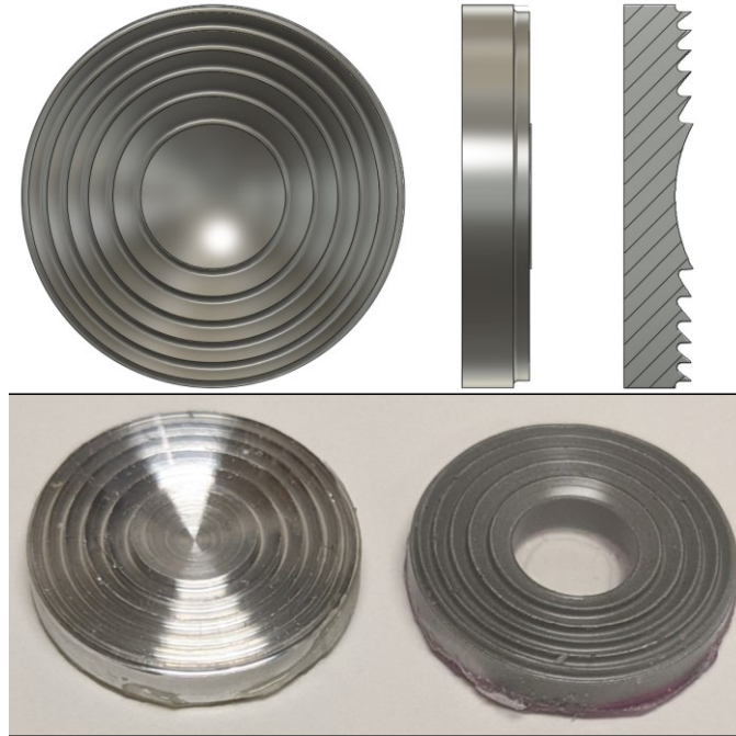
Figure 6.2: Top, side, and cross-section renderings of the final lens design are shown along the top, where the cross-section shows six separate surfaces. The bottom left and right images show the final machined Fresnel lens, both without and with a hole for co-registered imaging.
