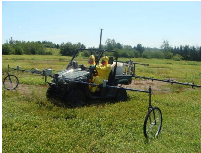
Fig. 2.1: Automation in agriculture (variable rate sprayer; Esau et al., 2014).
