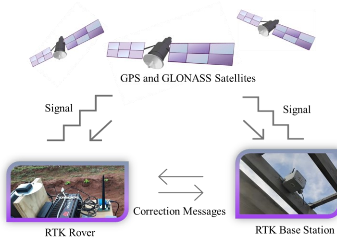
Fig. 4.11: The communication among RTK base station, RTK rover, and the satellites.
