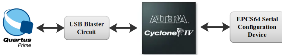
Fig. 4.5: FPGA configuration chain using Quartus Prime programmer.
