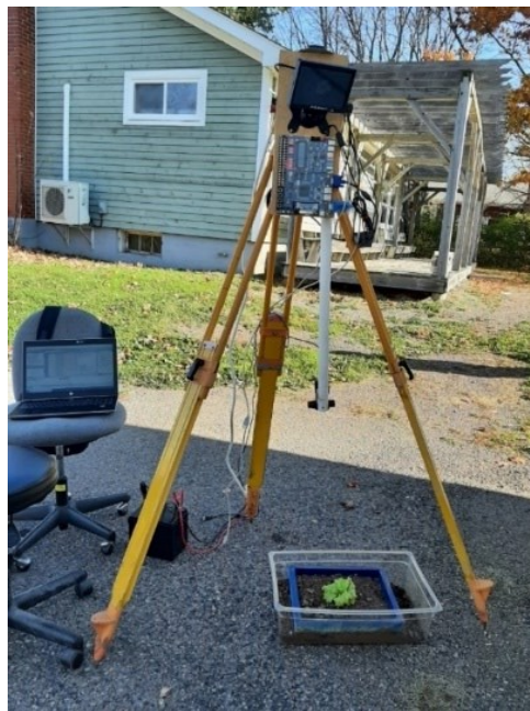
Fig. 4.16: Field data collection setup to validate RFIP system in the outdoor environment.
