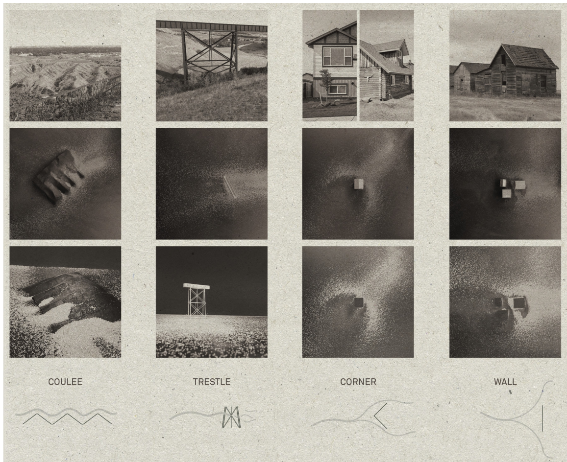
Wind behavior study of four typical forms found in the Lethbridge landscape: the coulee, the trestle, a building corner, and a building wall.
