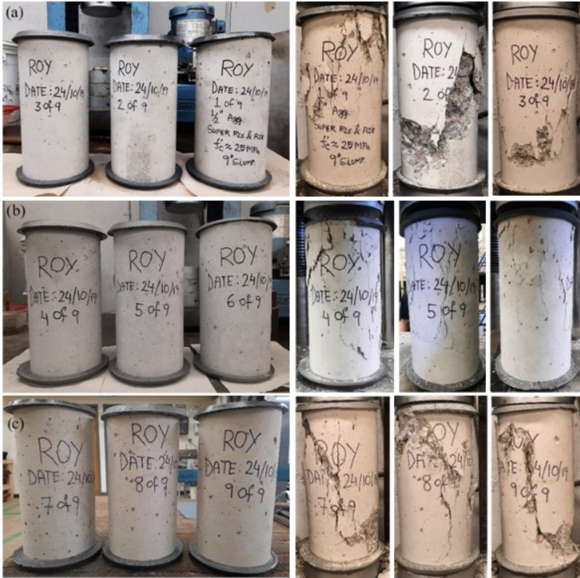
Figure 3-3. Three stages of concrete compressive test: (a) Initial; (b) Intermediate; (c) Final
