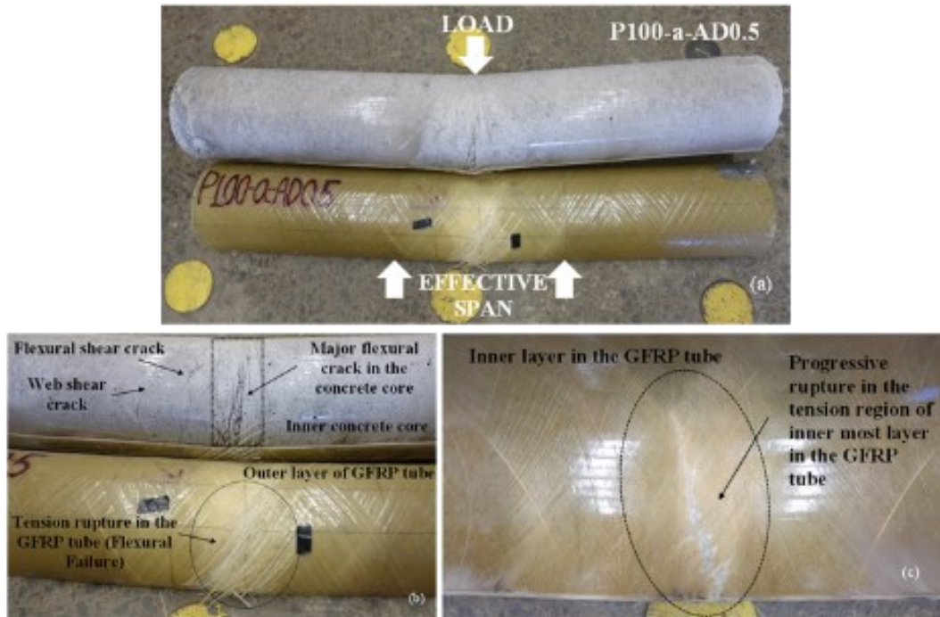
Figure 3-15. Failure modes in P100-a-AD0.5 specimen: (a) Longitudinal cross-section of CFFT; (b) Inner concrete core and outer layer of GFRP tube; (c) Inner layer of GFRP tube
