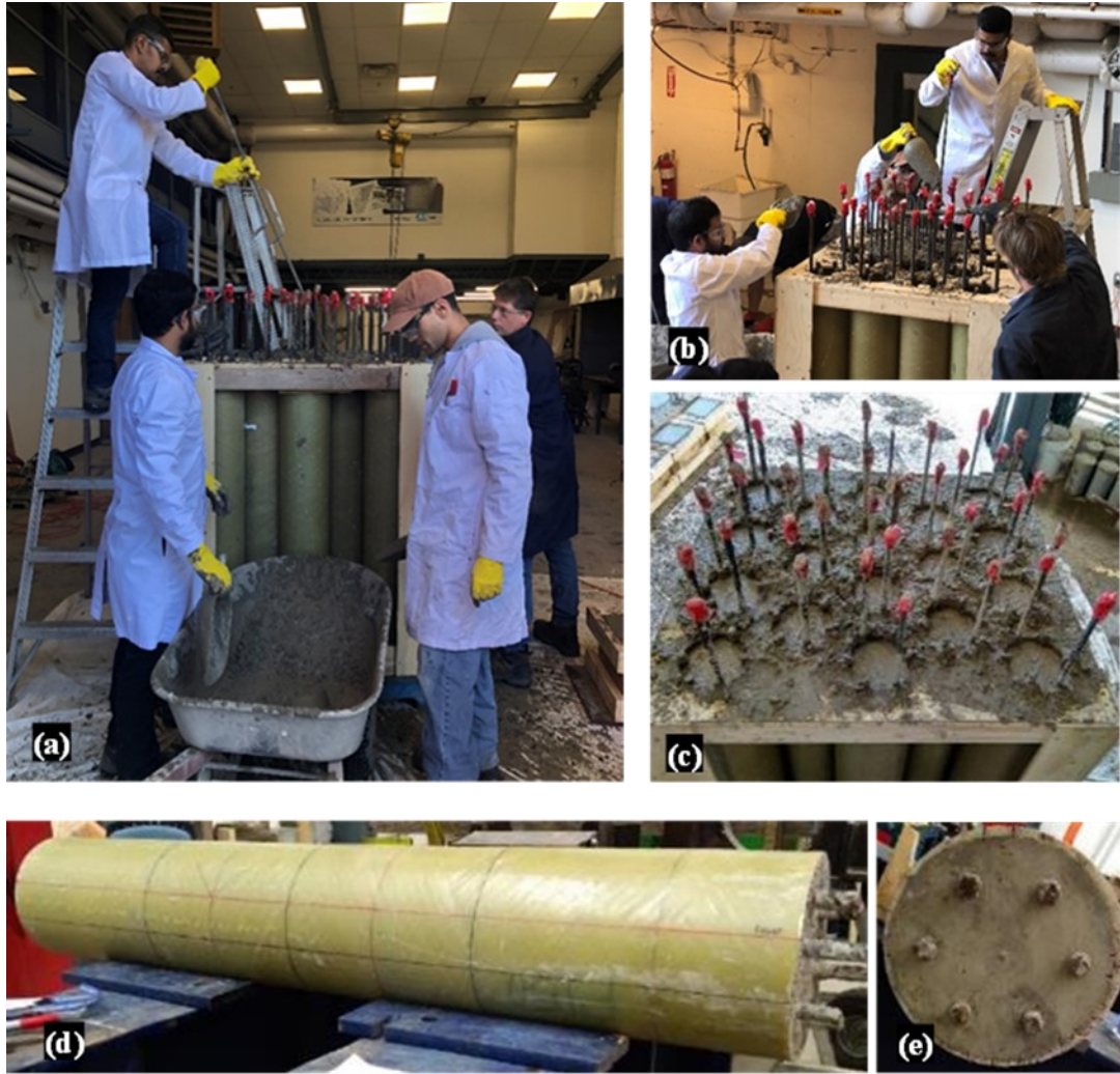
Figure 3-9. CFFT specimen casting: (a) Concrete pouring; (b) Concrete compaction during specimen casting; (c) CFFT specimens ready for curing process; (d) Longitudinal view of CFFT; (e) Cross-sectional view of CFFT
