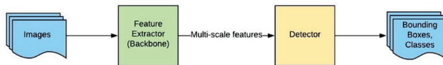
Figure 3.6: Overview of Yolov3 architecture [94]
