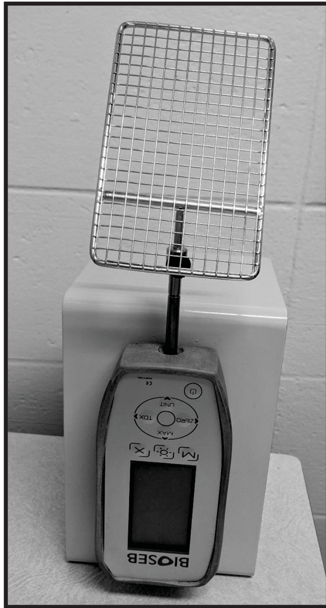
Figure 2.3.1: Instrument for measuring grip strength. Mice use their forelimbs to hold onto the metal mesh while being held upside down by their tail. Mice are gently pulled upwards, horizontal to the mesh. This process is done 4 times per mouse per timepoint. Grip strength is shown on the display in Newtons, as the highest force achieved for each pull.
