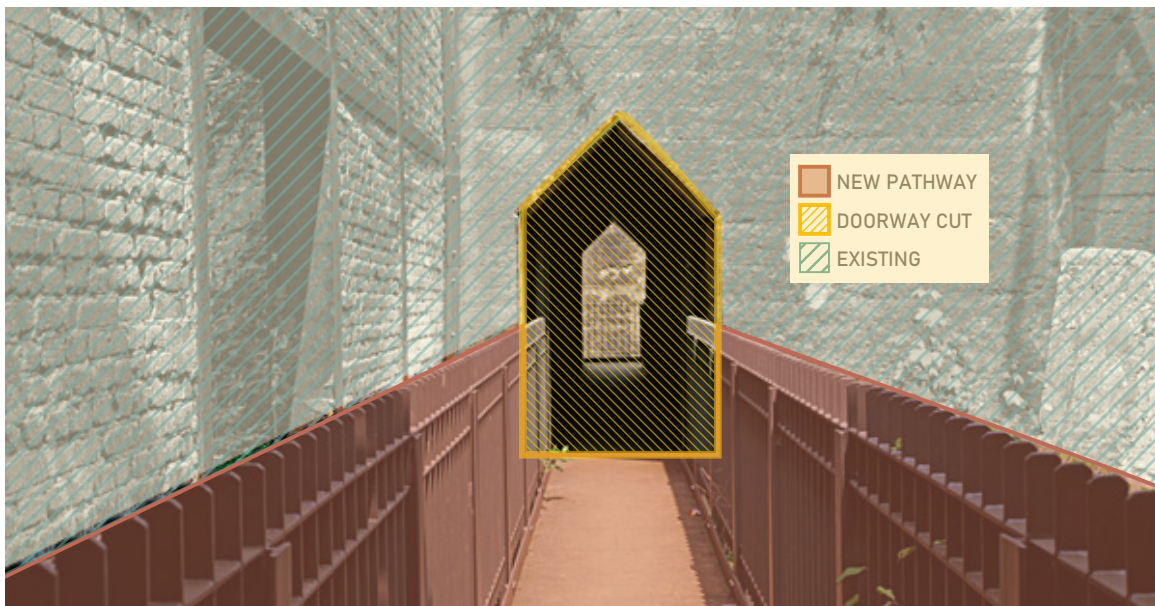
Diagram shows where existing structure has been modified to create new program at Landschaftspark. (Latz 2011)
