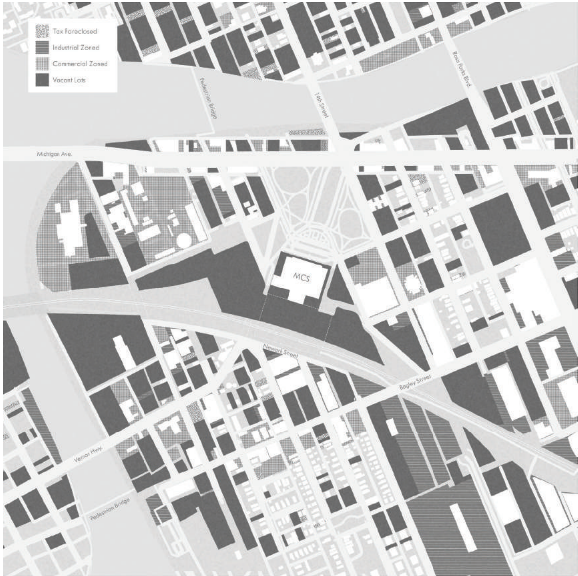
Site drawing showing the amount of industrial, commercial, and vacant lots around the station
