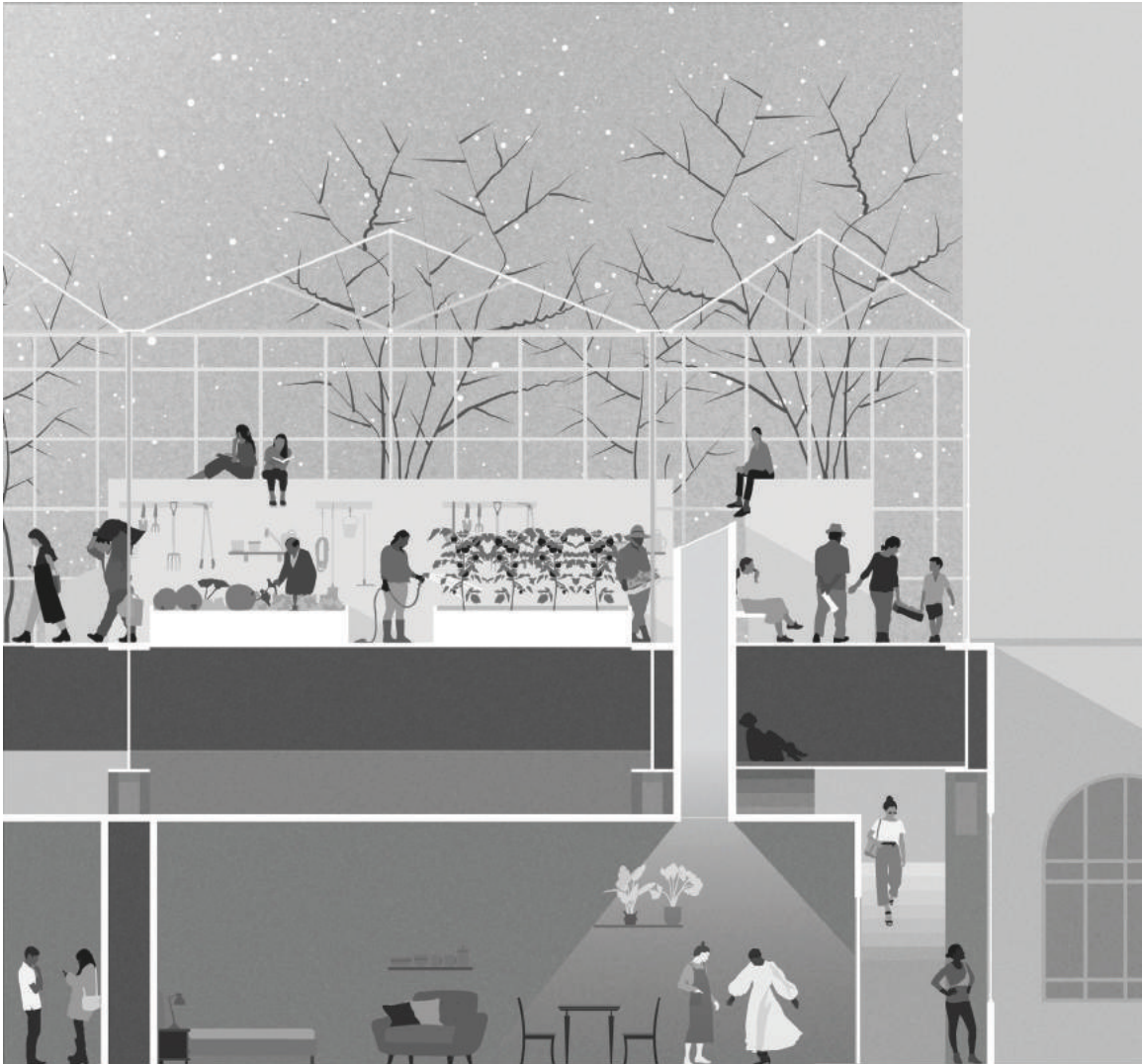
Greenhouse and undercarriage section. Residential treatment rooms are connected to the greenhouse through lightwells along what was once the platforms to the trains
