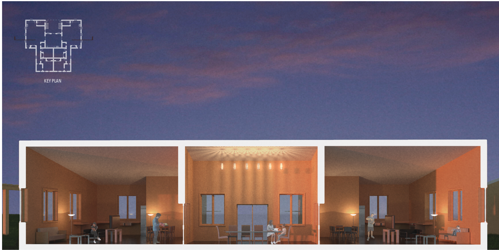
Perspective section of one of the housing buildings, showing the shared dining room and kitchen at the center of two units
