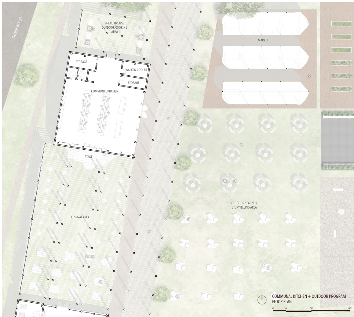
Floor plan of the communal kitchen and the outdoor program: festival area, outdoor cooking area, market, garden and storytelling area
