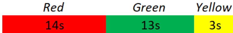
Figure 0-22 Reference Signal Cycle in Seconds
