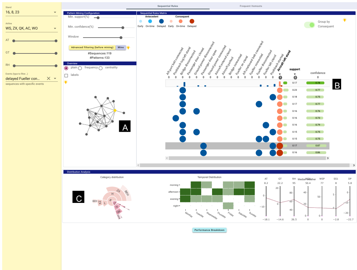
Figure 6.3: Target based analysis for delayed aircraft fuelling. Investigating Aircraft left stand patterns. (A) Target event is selected from the overview graph (yellow node). (B) The group with target event as the cosequent shows a dark orange bar in the corresponding cell, hinting a delay-related pattern. Group is collapsed and rows are sorted by support and confidence. (C) Attribute distribution for the selected pattern.
