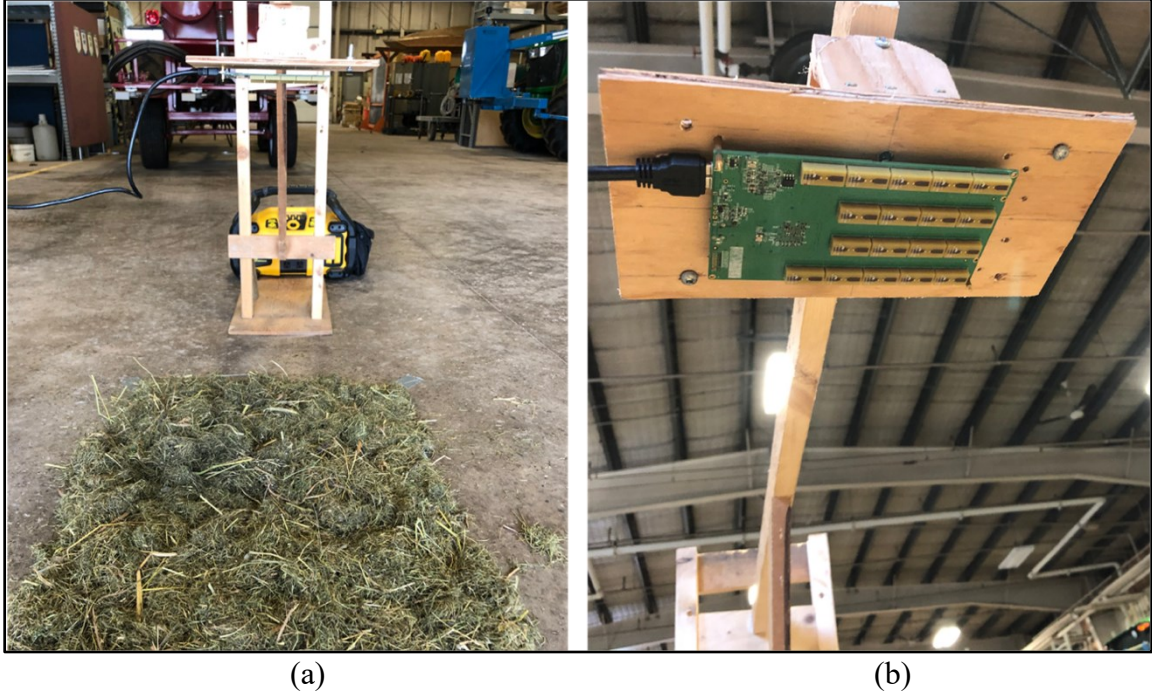
Figure 2-11: The Walabot radar trial with Wood/Grass clipping (W/G) treatment (a) and mounting socket (b) on mounting plate.
