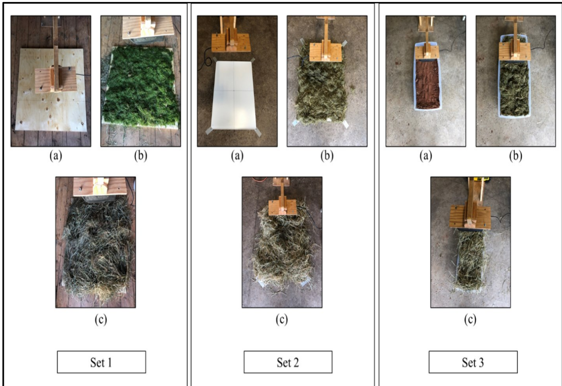
Figure 3-3: Experimental sets: Set 1) wooden boards as ground surface; Set 2) metal sheets as ground surface; Set 3) soil samples as the ground surface.
