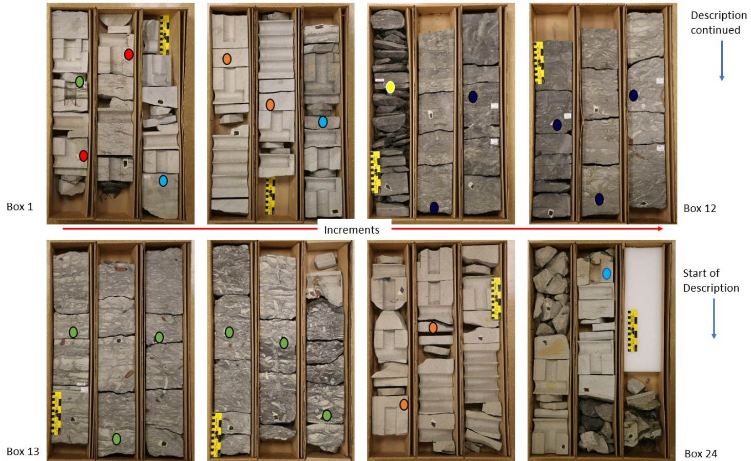
Figure A.1.2: Photo compilation of slabbled core from the Thebaud I-93 well's core No. 1 (3065.68-3081.27 mRT MD). The blue arrows indicate the flow of the core description generally from right to left and top to bottom of each box. The red arrow is generally indicative of the increment in box number from left to right. Small white square tapes with black shadings indicate the point where X-ray fluorescence XRF measurements were collected for rock classifications according to Herron (1988). The colored ovals represent the sand class facies distribution from our analyses. Green represents the litharenite, red for Fe-Sands, yellow for shales, orange for subarkose, dark/navy blue for wackes, and light blue for sublitharenite.
