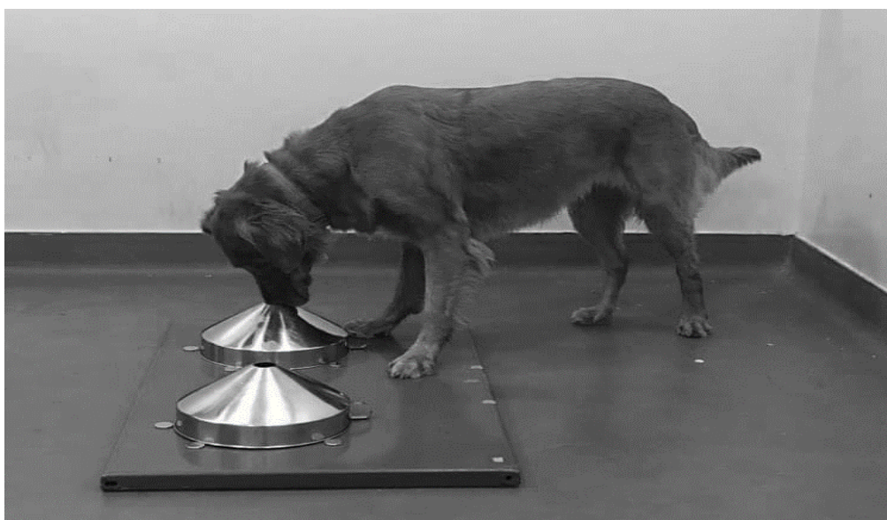
Figure 3: Glass scintillation vials containing a silicon-oil coated cotton ball and tea sample were placed beneath a metal funnel. The dog was asked to indicate a positive sample with a 5-sec nose hold
