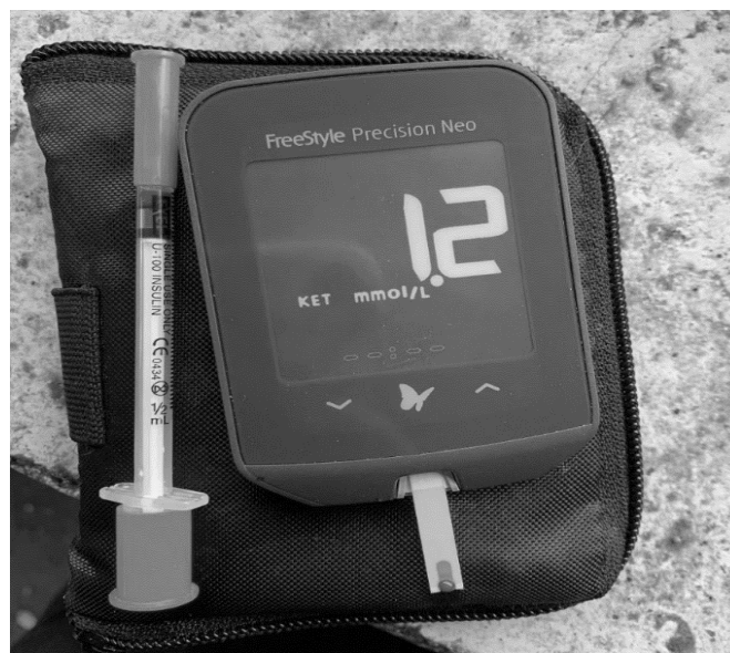
Figure 1: A Precision Xtra™ meter used to monitor the blood ketone concentrations of the cows at the Ruminant Animal Centre on days 7, 14, 21 and 28 post-parturition. A cow positive for ketosis will have a blood ketone body concentration > 1.2 mmol/L
