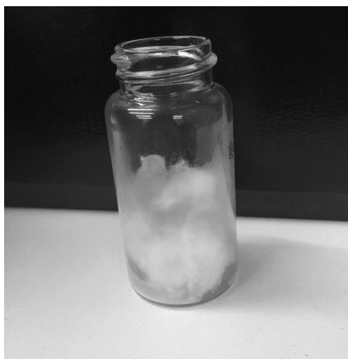
Figure 2: A 20 mL glass scintillation vial containing a silicon oil coated cotton ball was used for collection of breath from dairy cows positive and negative for ketosis
