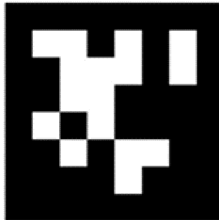
Figure 4.2: Example of a tag from the AprilTag fiducial tagging system [28] © 2011 IEEE.
