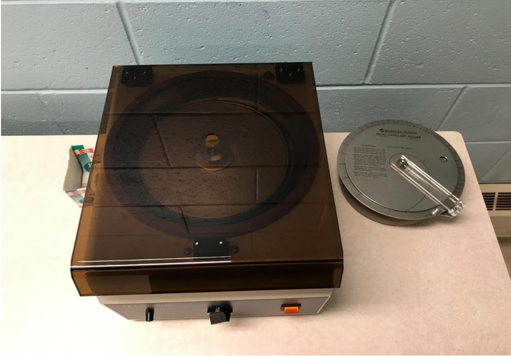
Figure A4.1 Centrifuge and hematocrit reader used for packed-cell volume test
