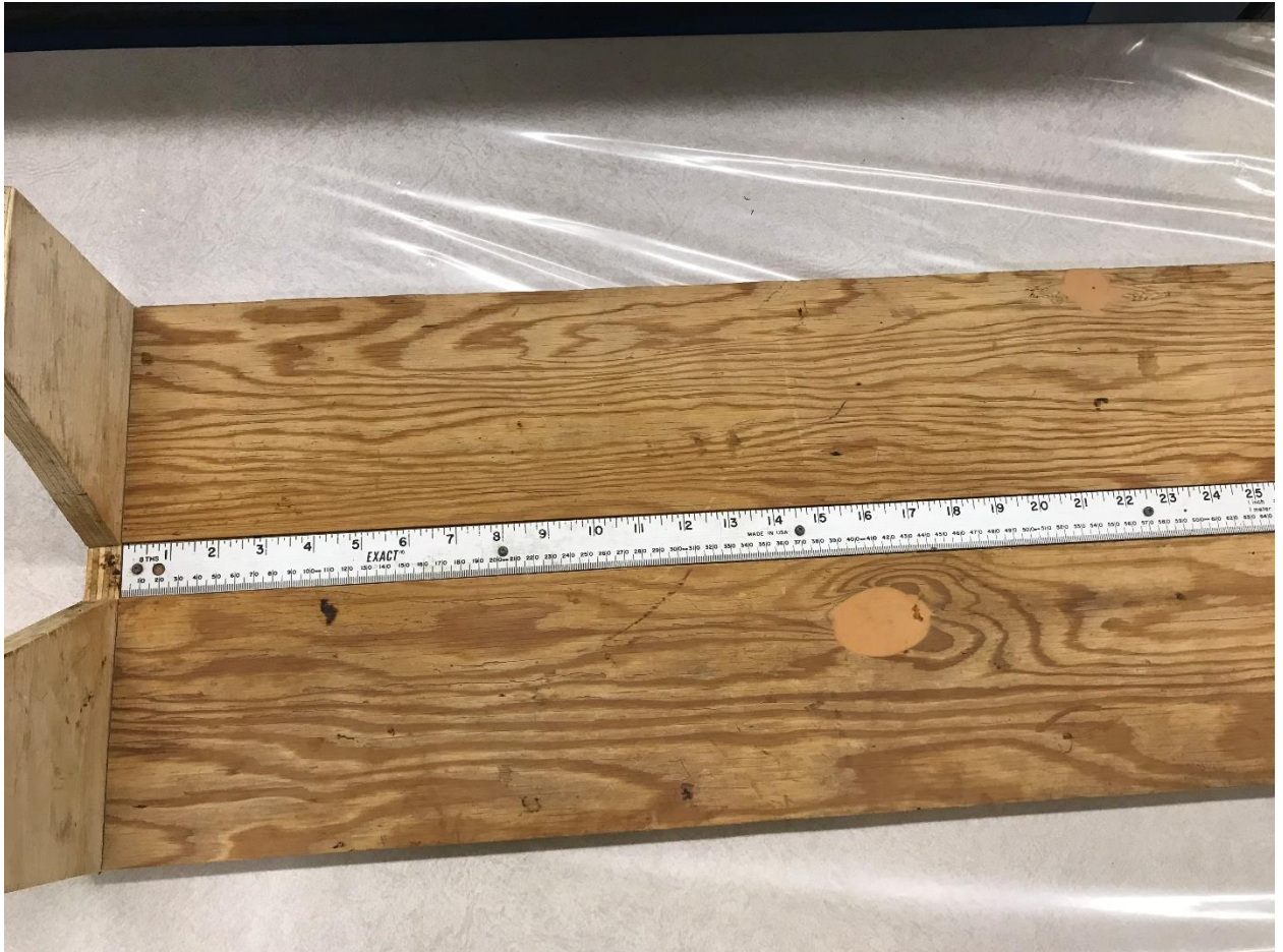
Figure A5.1 The measurement board used to measure the harvest body length of mink
