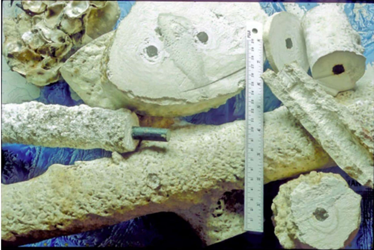
Figure 4. Biorock material grown in the Maldives. Photo by Wolf Hilbertz (mtessis, 2018).
