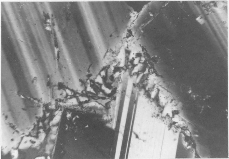
Figure 35 Reaction zone around a plagioclase crystal. Photo taken with crossed nicols. Magnification, 130X.
