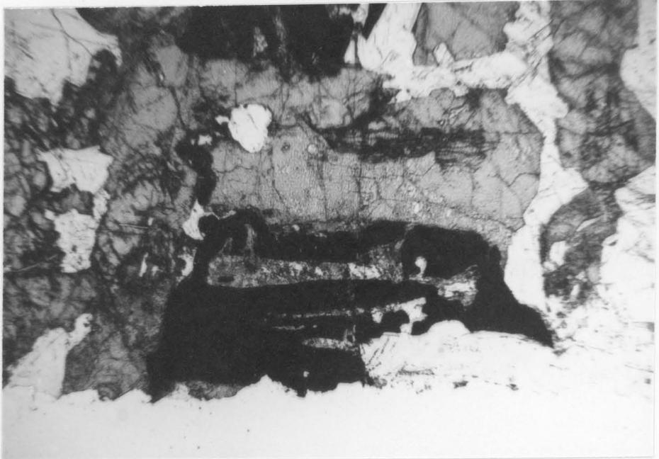
Figure 36 Large skeletal crystal of magnetite. Photo taken in plane light. Magnification, 20X.
