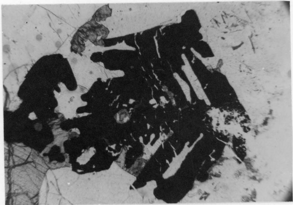
Figure 37 Large skeletal crystal of magnetite with intergrown ilmenite. Photo taken in plane light. Magnification, 20X.
