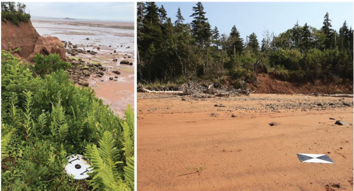
Figure 2.4.2: Left: semi-permanent GCP in the form of a plastic bucket lid held in place with landscaping staples and ½ inch rebar near the cliff break. Right: Coroplast™ GCP target in place on the beach at Thomas Cove.
