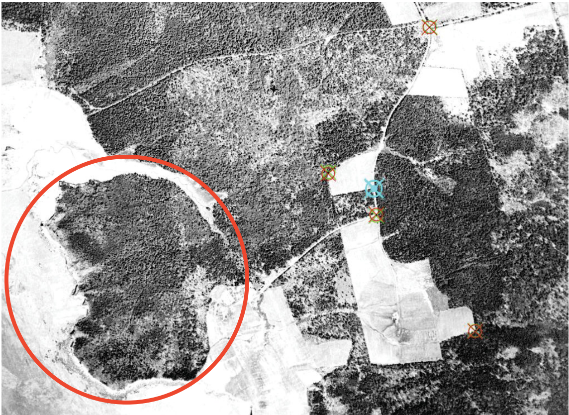
Figure 2.2: Study site is circled in the bottom left of the frame. The position of 5 control points are shown over an image from 1938. These control points were used for georeferencing the historic air photo against features still clearly visible from modern aerial imagery, such as road intersections and field corners. Notice that the 5 control points are all located to the east of the cliff and are roughly collinear.
