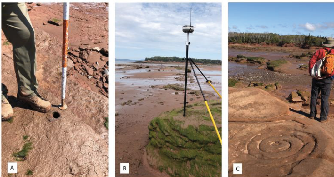
Figure 2.4.1: A) borehole used as a checkpoint on the south end of the cliff. B) same borehole as in panel A with bipod rover mast in place. C) large spiral petroglyph used as main localization point near the middle of the cliff. This feature, which is on top of a large outcrop that is easily accessible, is situated in the middle of the survey area both horizontally and vertically.
