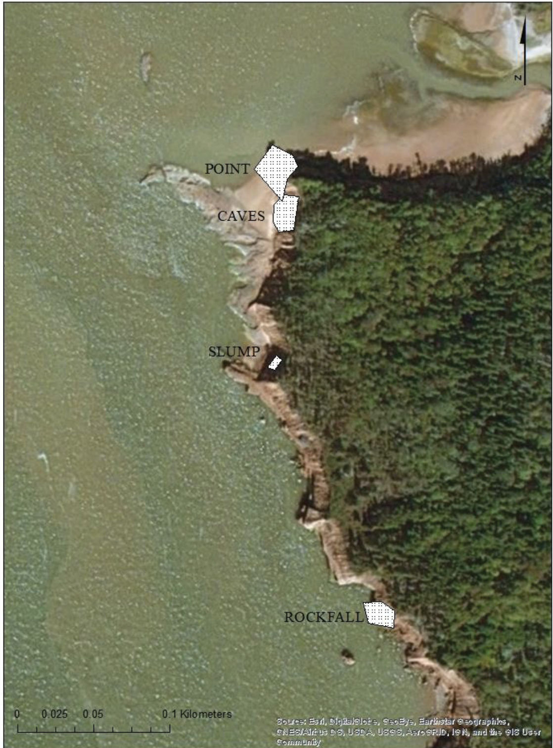
Figure 2.8.1: Polygons used for volume calculation within Pix4D. Sites were selected based on visual observation of change and representation of typical shoreline features.
