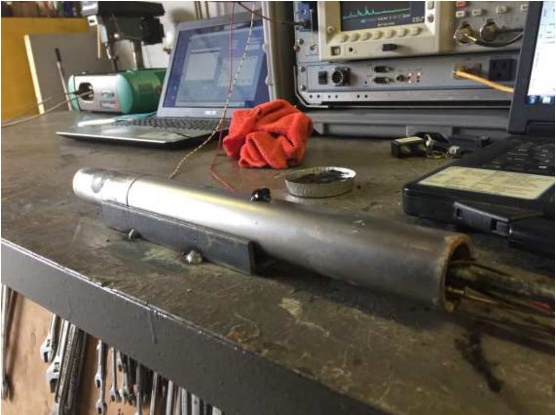
Figure 21: Preliminary UVOST trials on a BEIS sample. The sample is placed atop the UVOST probes sapphire window, from which, UV light is emitted.
