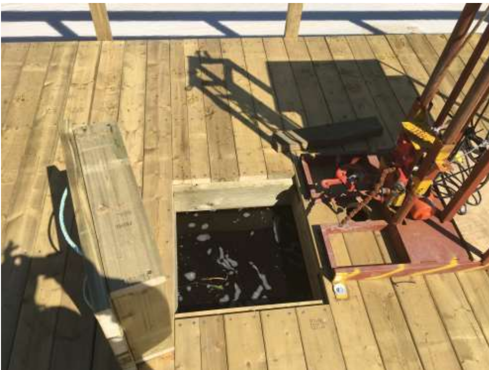
Figure 27: Field trails barge sampling sites for sediment gravity coring (left) and UVOST probing (right).
