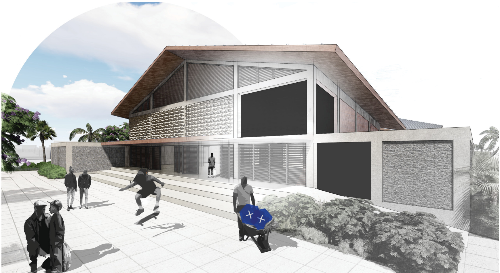
Rendered view of the Workshop from the courtyard. Panel infill can comprise suitable materials that will allow for shading and ventilation. Shown on the upper level is an infill reclaimed halved buckets. The Workshop is represented as unfinished, with the framing system drawn over the imagery and with wall panels missing to indicate that ultimately, the Co-op is the designer and I only provide the framework within which they work.
