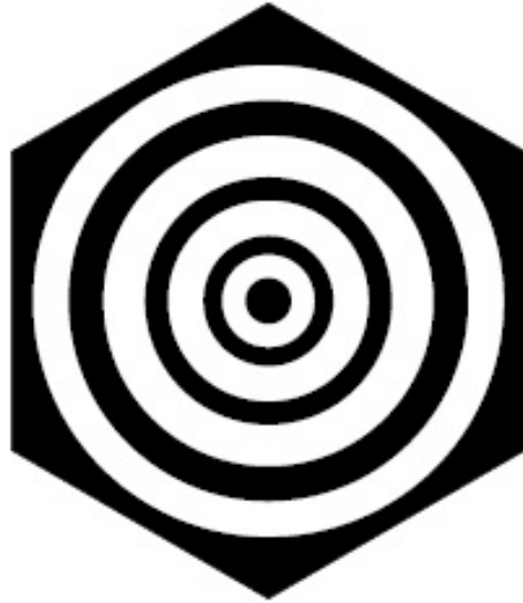
Figure 2.4: Landing target proposed by Lange et al. to reduce the dependence on full target detection. While the UAV no longer needs to have the entire target in its line of sight, it still requires good visibility and must land on the target. Reprinted with permission from IEEE © 2009 [35]
