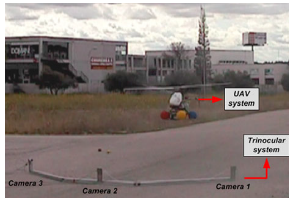
Figure 2.5: Ground-based stereo vision position estimation as shown by Martinez et al. The UAV vibrations are removed from the pose estimate at the cost of accuracy. Landing targets are no longer required, however line-of-sight is. Reprinted with permission from Springer Nature © 2011 [21]
