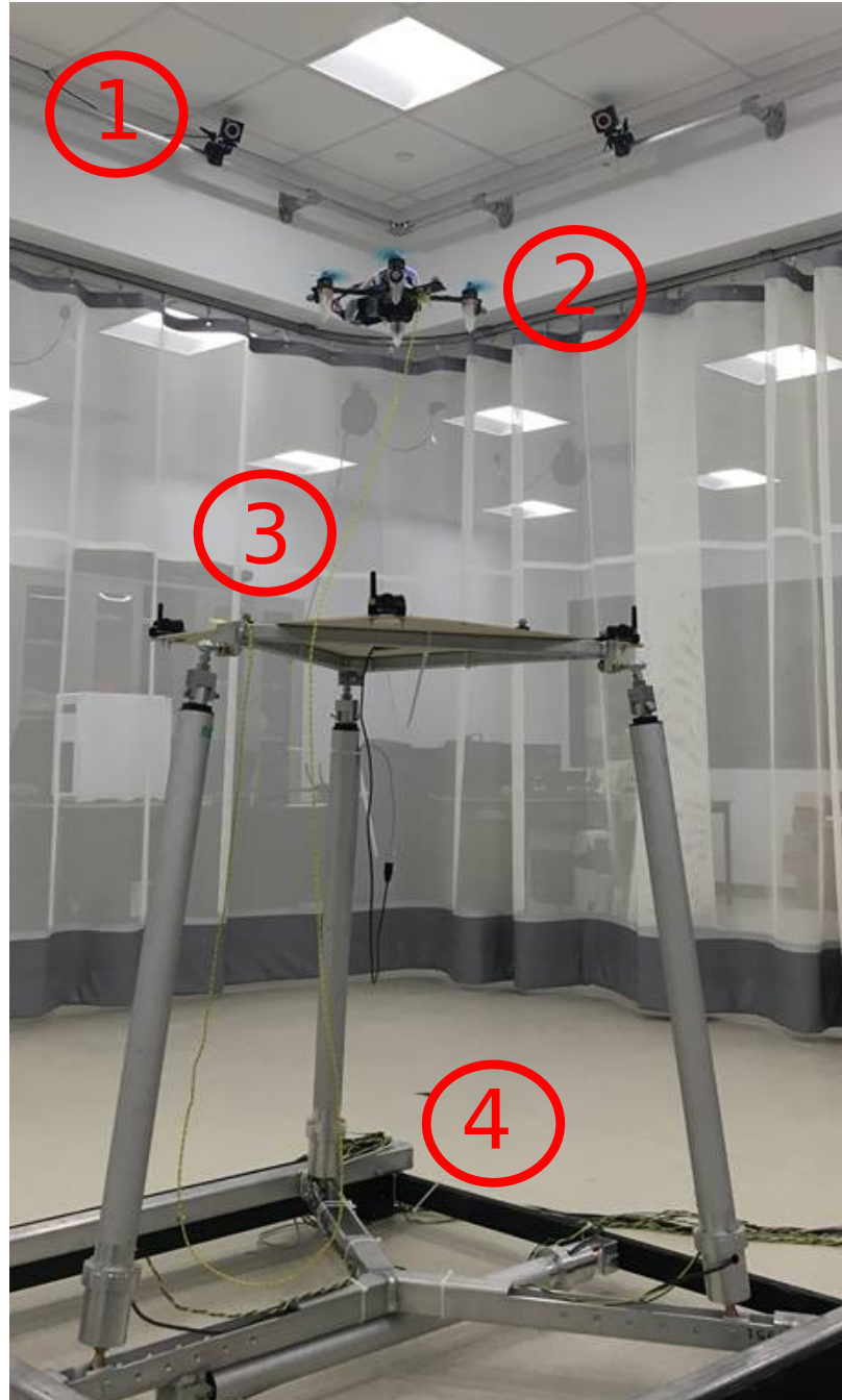
Figure 5.7: Hardware experimental environment within the ISL flight space: 1) Motion capture cameras (2 of 8). 2) Drone. 3) Acoustic sensors. 4) Stewart Platform
