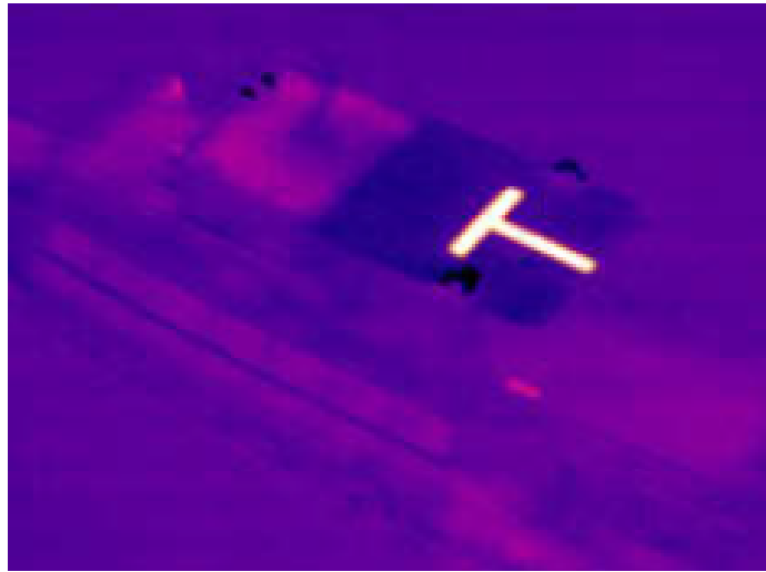
Figure 2.8: Infrared landing target as shown by Xu et al. They improved the pose estimate accuracy for IR however returned to requiring special landing pads. Reprinted with permission from Elsevier © 2009 [54]
