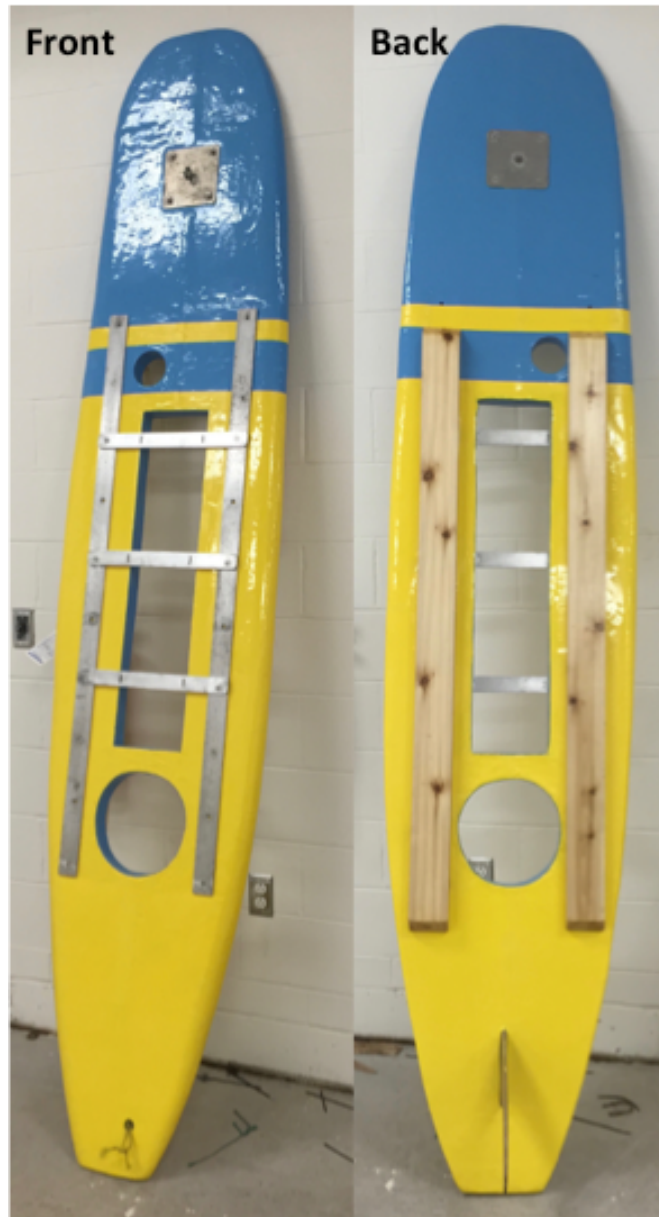
Figure 3.2 Completed surfboard-surface-vehicle, including front view (left) with aluminum flatbar, and back view (right) with cedar skids.
