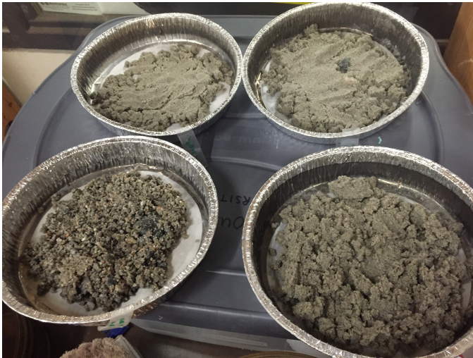
Figure 3.8 Sand samples obtained from varying water depths including: onshore; swash zone; 1.5m; and 3m. Samples were washed and left to dry in aluminum pie tins lined with coffee filters in preparation for sieving.
