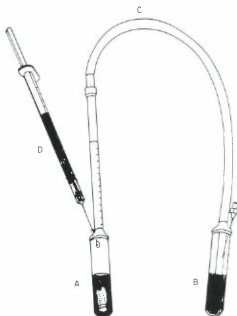
Figure 1. An apparatus for separation between carbonate and organic matrix from small pieces of coral skeletons (see text for further details).
