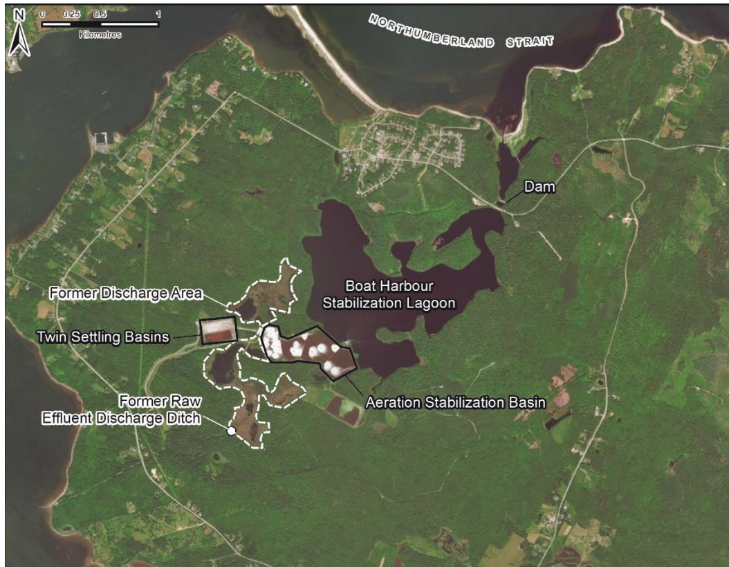
Figure 31: Components of the Boat Harbour Treatment Facility, including the original infrastructure (1967 - 1972) and the upgraded treatment facility (1972 - present). [Map produced using ArcGIS®].
