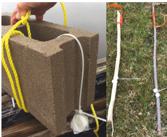
Figure 19: Left - DGT disks attached to a brick using a zip tie. This deployment method was used for DGT 1 and DGT3 (deep wetland samples), and DGTs in BH. Right - DGTs attached to posts. DGTs were deployed using this method for shallower wetland samples (DGT 2, 4-10), and in the dry cove.
