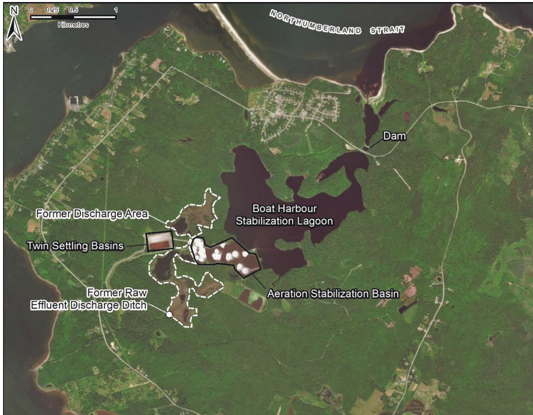
Figure 2: Components of the early treatment framework (1967 – 1972) and the current treatment framework [Map produced in ArcGIS®].
