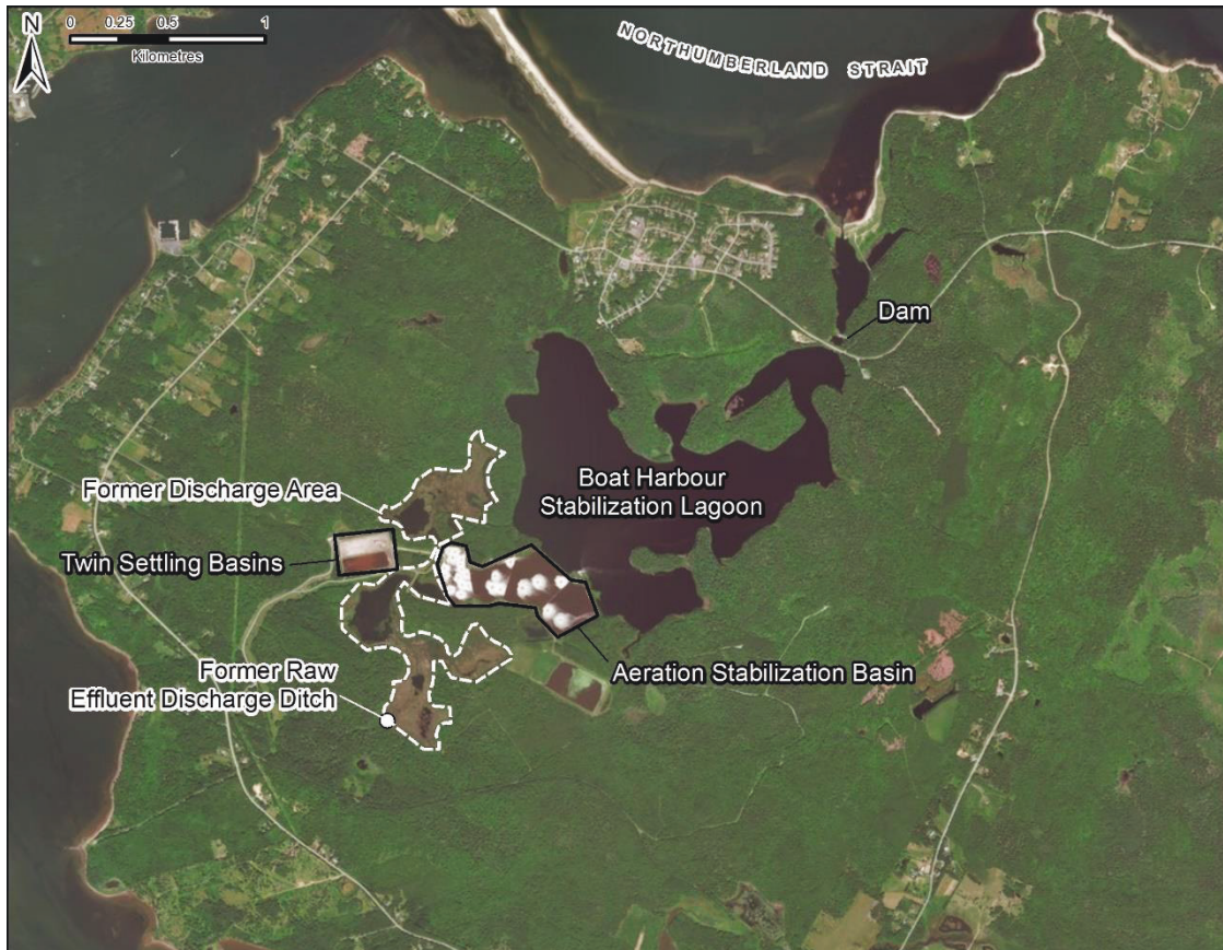
Figure 13: Components of the early treatment framework (1967 - 1972) and the upgraded treatment framework (1972 - present). [Map produced in ArcGIS®].
