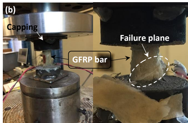
Figure 2. FRP material properties: (a) stress-strain behavior in tension and compression; and (b) GFRP bar compression test.
