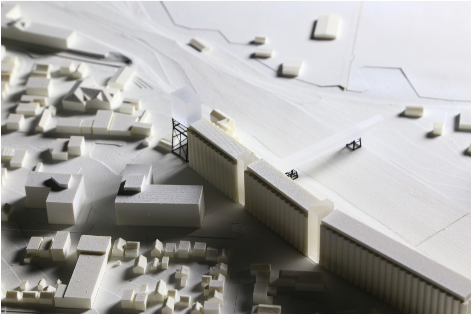
Site model photo showing the residential neighborhood is hiding in the shadow of the high silos' body and lacks sunlight in the morning until early afternoon.
