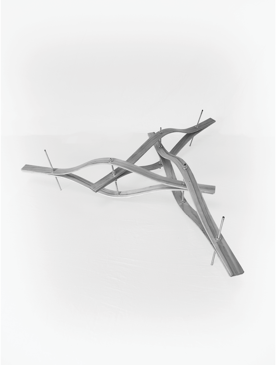
Scale model of a section of the steam bent wooden structure. Steam bending is a tactic used frequently in wood boat building as it enables wooden members to be formed around a ship's hull. Metal rods fasten the steam bent pieces together while simultaneously providing anchor points for possible textile cladding and connection to the ground.
