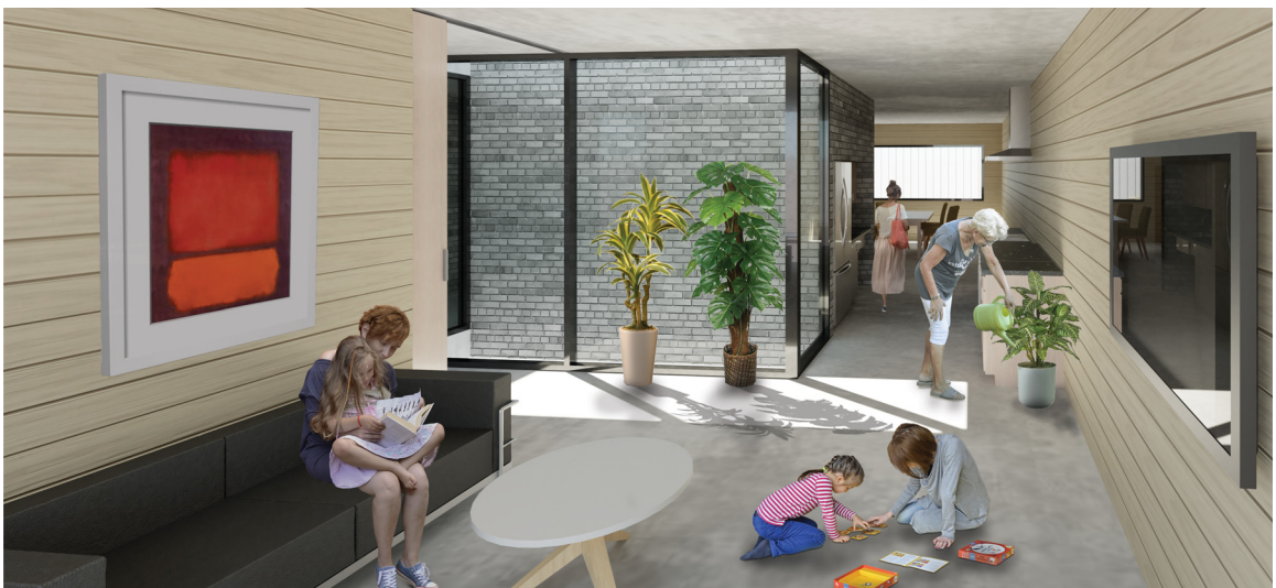
Figure 58. View of how a skylight provides light to a block housing unit's living room and kitchen.
