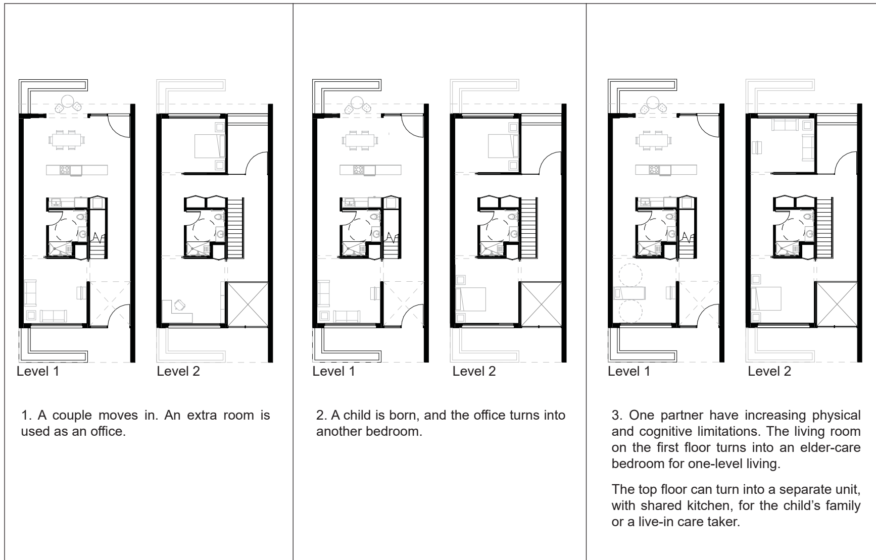
Figure 61. Diagram of how a typical unit in a row housing typology adapt throughout a person's life course.
