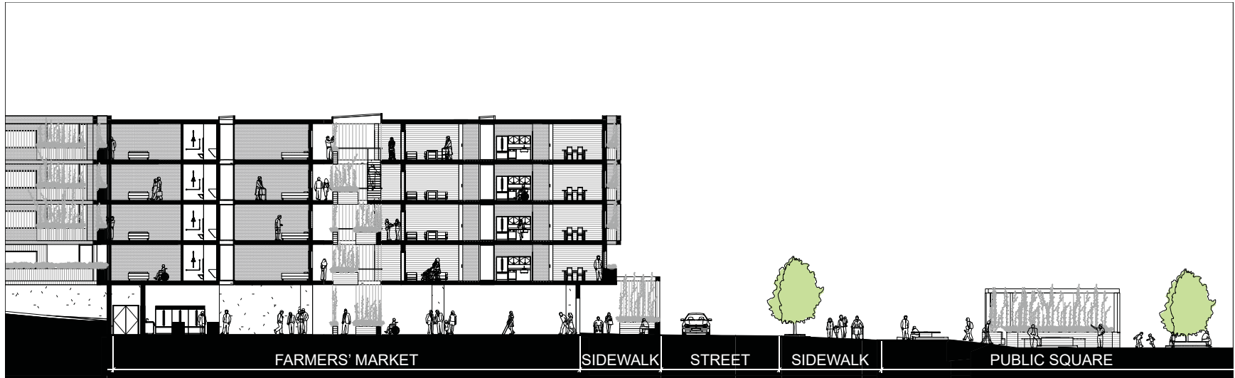
Figure 53. Section A - Block housing site section showing its relationship to the public square.
