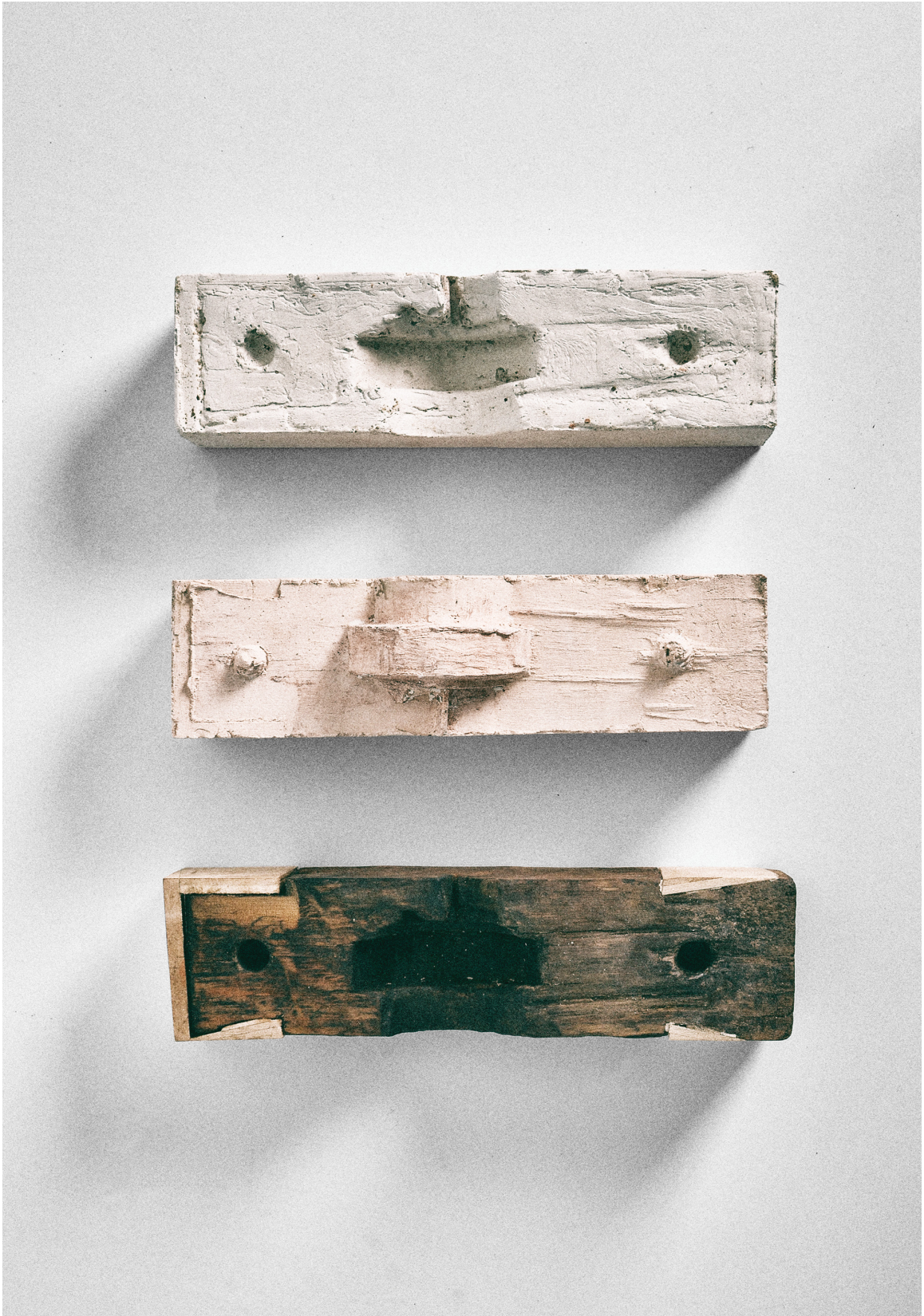
Models showing the casting process. Step 1 (bottom): an existing artifact made "whole" with new wood intervention. Step 2 (middle): negative cast of step 1. Step 3 (top): recast positive of step 2.
