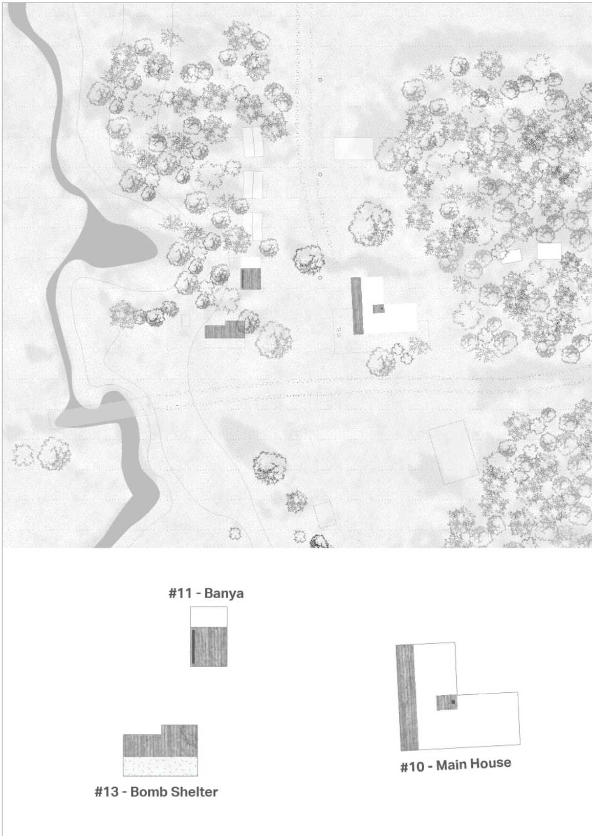
A site map of Homestead T53R9 Section 21, showing the 3 proposed sites for an intervention: #10 Main House, #11 Banya, #12 Bomb Shelter. The concrete textured hatching indicates the areas of each building that I will use a casting method to intervene.
