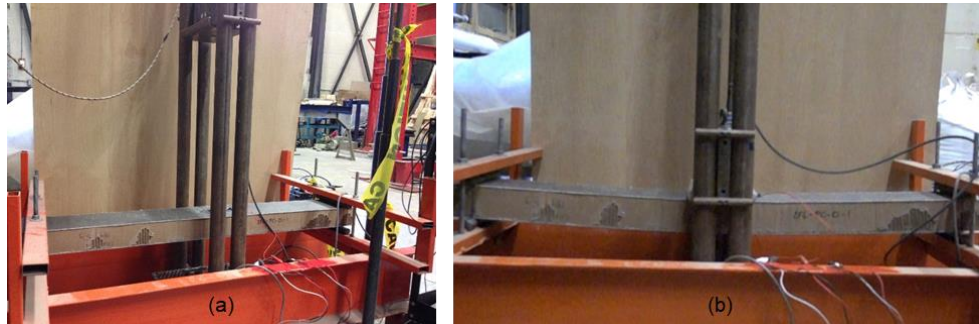
Figure 4. Impact Test (a) Set-up (b) Impact Event
