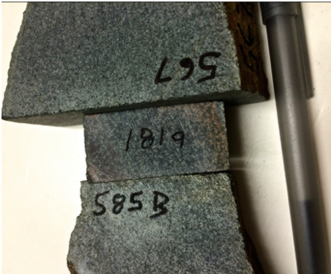
Fig. 6.10 Claremont sample 1819 (representative of mafic species) appears identical to DNR basalt samples 12TM0567 and 12TM0585B from the Byers Brook Formation. BIC pen for scale.
