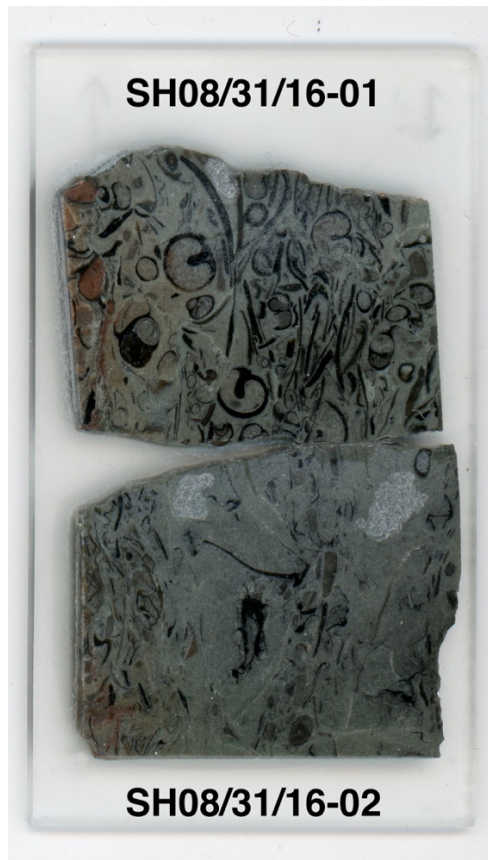
Fig. 3.4. An example of a polished standard size slide with samples collected from the upper Stonehouse Formation, Arisaig, Nova Scotia. Sample numbers are written above and below the samples. Various shelled organisms are visible in the specimens.
