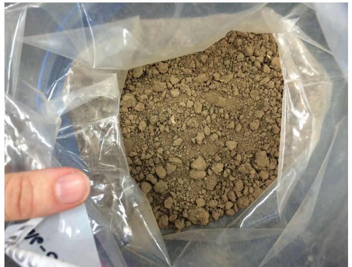
Figure 22: (b) Open bag for soil to air dry
