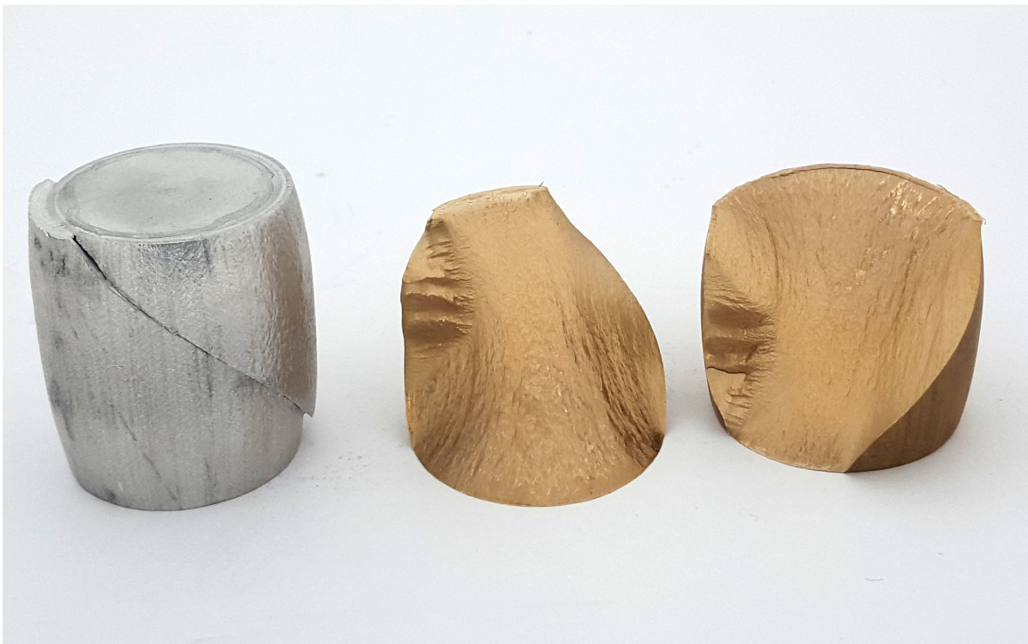
Figure 5.2: Fractured aluminum (left) and the two halves of a fractured brass specimen.
