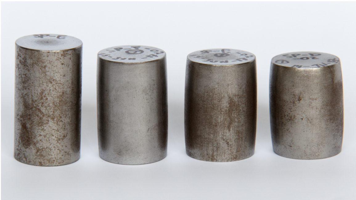
Figure 6.1: SP-4420 specimens of all three densities (decreasing to the left) after testing compared to an untested specimen (far left)
