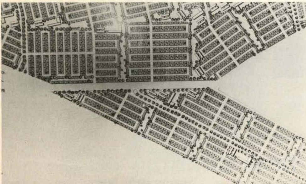
.....The 1/80" scale plans were assembled on a base map and reduced to 1/200". Above is a close-up of plan at 1/200" scale
