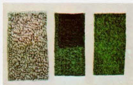
Nylon 100 hours Polypropylene without stabilizers 216 hours Polypropylene with stabilizers Over 2,000 hours
