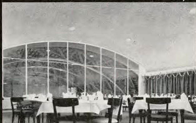
The dining room of a Toronto gentlemen's Club has an Asbestospray ceiling for acoustical correction. Architect: Basil G. Ludlow, Toronto General Contractor: W. B. Sullivan Construction Ltd. Toronto Asbestospray by: David McFarlane & Assoc. Ltd. Toronto.
