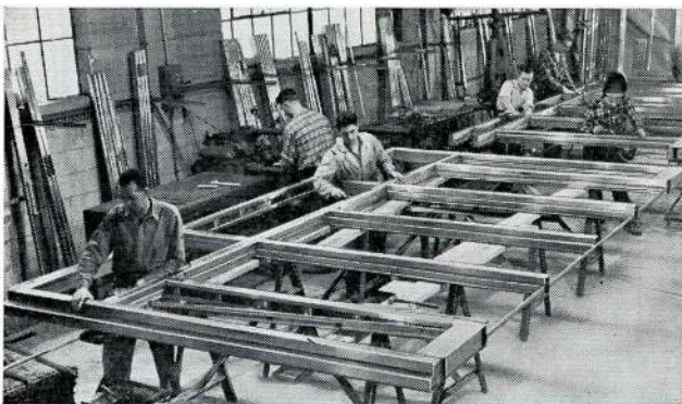
Chubb Craftsmen weld the doors to form one complete unit
