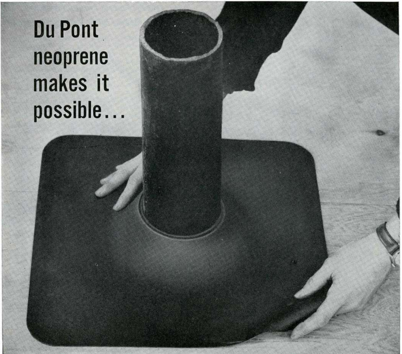
Special double-seal collar design assures weathertight fit on one-piece Carlton "Mono-Flash" Neoprene Roof Vent Flashing. Finish material can be applied right over flashing's broad apron and up to base of collar. Du Pont neoprene synthetic rubber assures long life for flashing.
