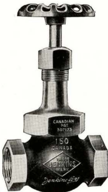
Fig. 106-A—Standard Bronze Globe Valve for 150 lbs. working steam pressure or 250 lbs. oil, water and gas working pressure. Has special exclusive Jenkins features, including one-piece screw-over bonnet and slip-on, stay-on disc holder.
