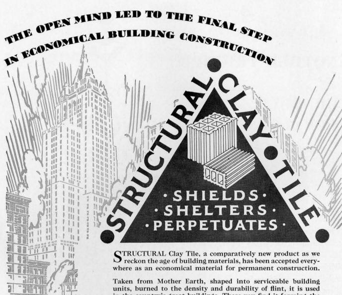
Taken from Mother Earth, shaped into serviceable building units, burned to the density and durability of flint, it is used in the country's great buildings. There you find it forming the walls, the floors, the partitions, and fireproofing the steel work. Never have the quality, variety, and availability of Structural Clay Tile been so marked as they are today. There are shapes and sizes for every building need.
