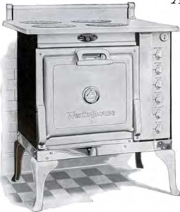
Type "HS-2", 4-element range: 2 1500-watt and 2 950-watt. Oven: 2 1200-watt elements. Floor Space: 30 \frac{1}{8} " x 24 \frac{1}{4} ". Duo-tone Porcelain Finish in white and grey vitreous enamel.
