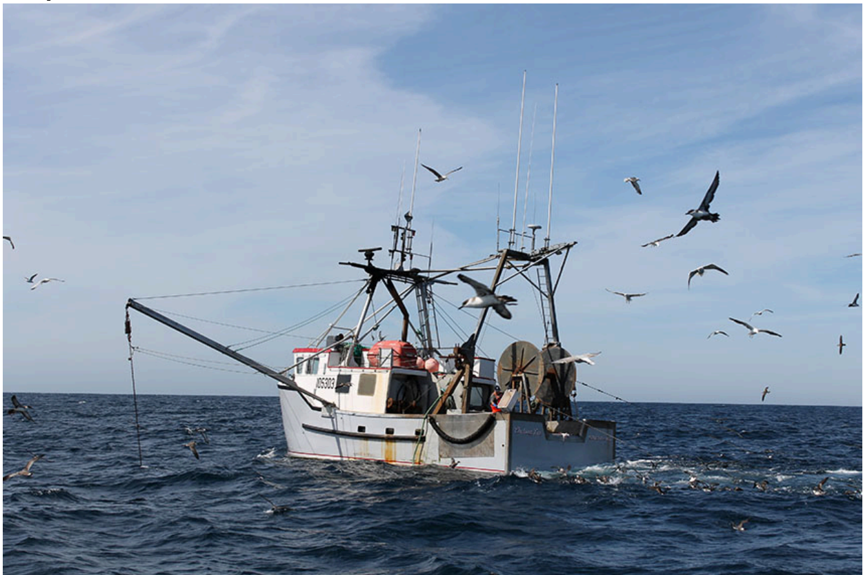
Image 14.3. Bottom-dragging is a technology used to harvest fish or scallops by drawing an open net along the sea floor, which in some respects is the marine equivalent of clear-cutting a forest. This boat is used to drag for scallops off southwestern Nova Scotia. Source: B. Freedman.
