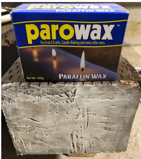
Figure 3.16: Creosote/ diluent treated rail tie after it was measured, cut, and then sealed with Paraffin Wax.
