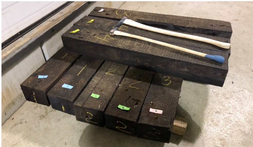
Figure 3.14: Rail ties used for rainfall simulation before they were cut to dimensions 100.3 cm x 15.24 cm x 20.32 cm.
