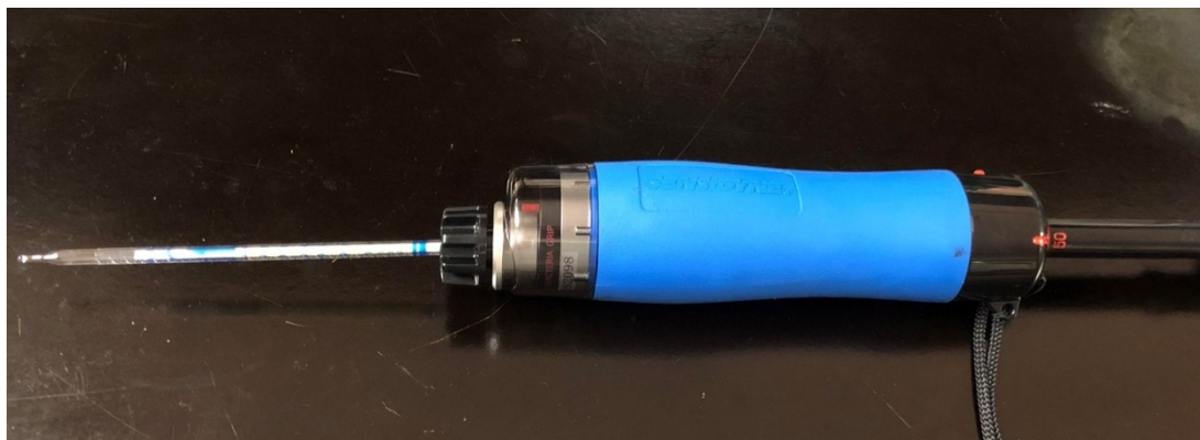
Figure 3.9: Colorimetric tube attached to pump to collect air samples of creosote.
