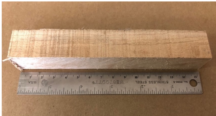
Figure 3.5: 25 cm x 15 cm x 15 cm block of wood used in pilot plant to simulate full scale production against 15 cm ruler.
