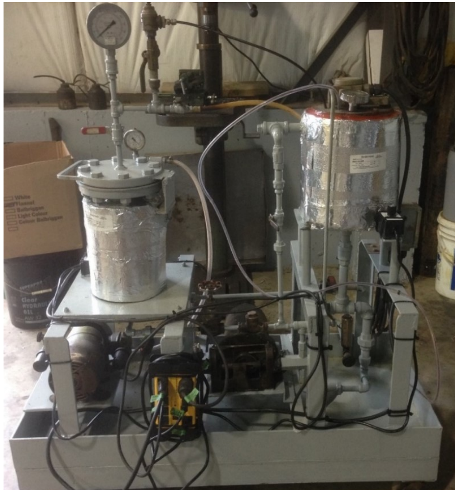
Figure 3.1: Pilot plant used to treat wood blocks as well as collect samples of liquids and gases.
