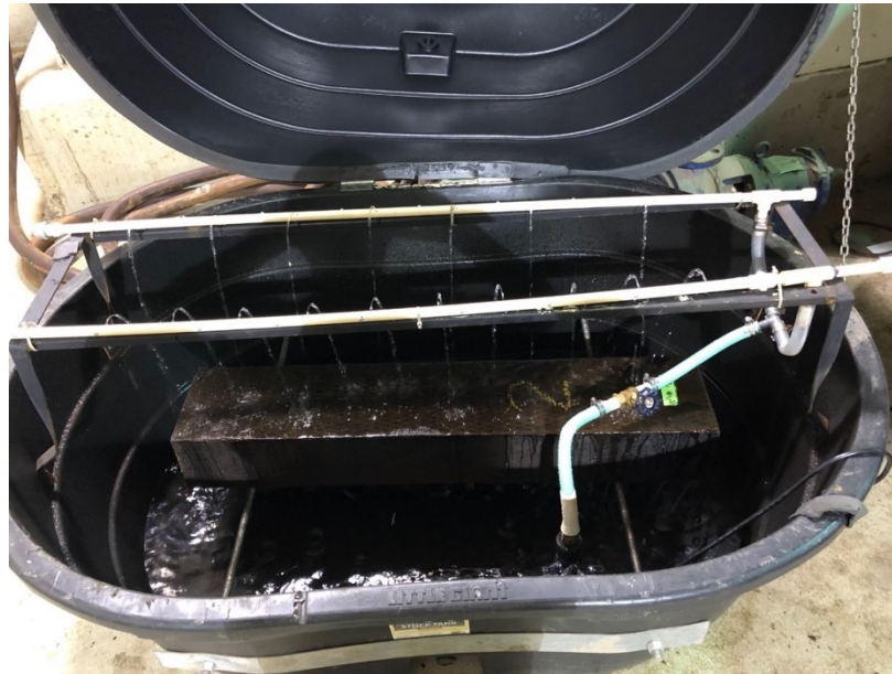
Figure 3.17: Rainfall simulator where the rail tie is sitting above the pool of water. In which case the water is being pumped through the PVC pipes and raining onto the wood sample.
