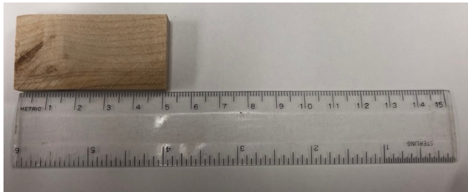
Figure 3.3: 50 x 25 x 7.5 mm Rock Maple wood block used for fungi trial against a 15 cm ruler.
