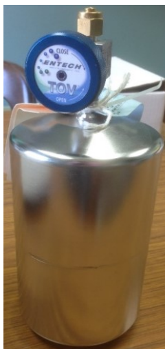
Figure 3.7: Summa Canister used to collect creosote gas samples for PAH analysis.
