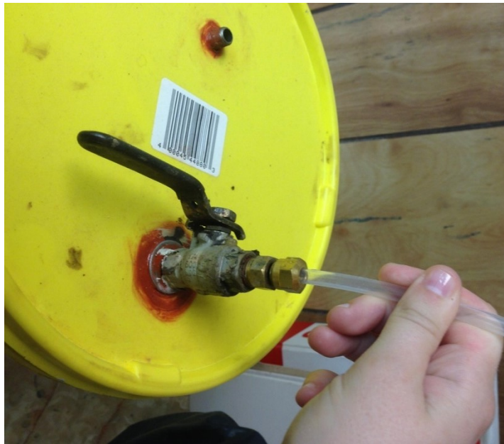
Figure 3.8: Valve attached to the lid of the 10 L bucket to collect samples using a Summa Canister.
