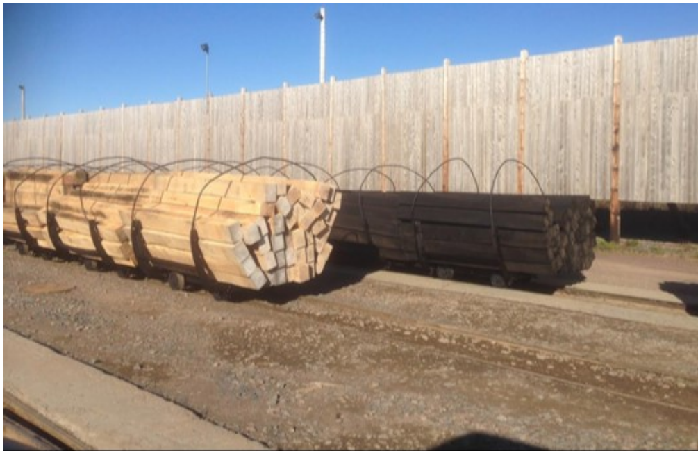
Figure 1.1: Photo of rail ties treated with creosote after preservative cycle, next to untreated ties at the Stella-Jones Inc., Truro Plant.
