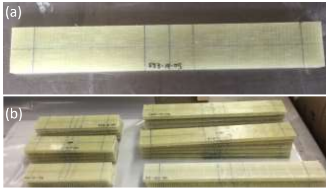
Figure 3. Fabricated specimens: (a) G1-S300 specimen; and (b) complete test matrix.
