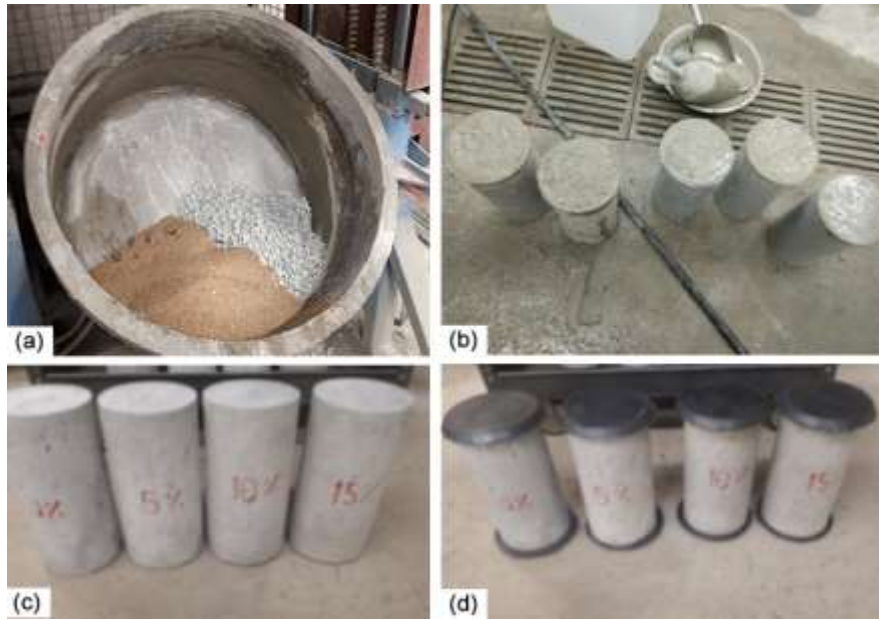
Figure 3: Preparation of concrete specimens: (a) mixing the concrete materials; (b) fresh concrete poured in the cylindrical molds; (c) concrete specimens after curing; (d) capped specimens
