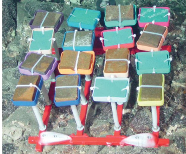
Figure 2.2: Array of larval settlement collectors at deployment in 2006 (South wall: 671 m). Collectors included either a basalt rock ( \sim 7 \times 10 \times 2 cm) supported by a plastic ring ( n = 10 ), or mesh pads ( \sim 7.5 \times 10 \times 1.5 cm, blue ‘Scotch-Brite’ pads, mesh openings: \sim 3.5 mm 2 ) ( n = 6 ).
